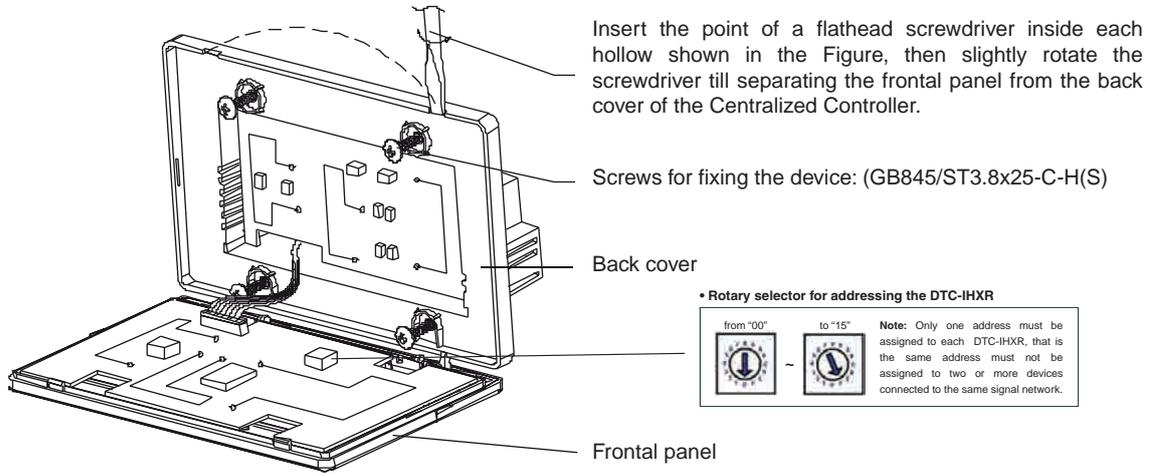
Detail of the terminal blocks and the contacts for the connection of DTC-IHXR
