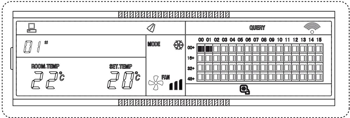
As already observed, each box of the grille is identified by a pair of coordinates, that is by the column and by row number the box belongs to. In the signal network of DTC-IHXR Centralized Controller, the address of each Indoor Unit is given by the sum of these coordinates. For example, for the Indoor Unit which appears in the box “00, 00+”, the address assigned in the signal network is: 00 + 00 = 00. The screen in “QUERY” Mode shown above gives the following information:
