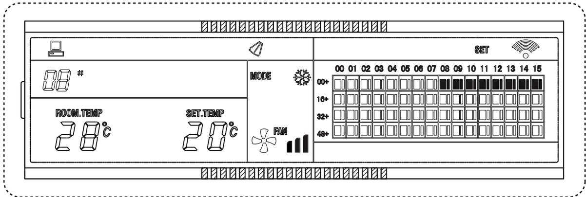
As already observed, each box of the grille is identified by a pair of coordinates, that is by the column number and row number which the box belongs to. In the signal network of DTC-IHXR, the address of each Indoor Unit is given by the sum of these coordinates. For example, for the Indoor Unit which appears in the box “08, 00+”, the address assigned in the signal network is: 08 + 00 = 08. The screen in “SET” Mode shown above gives the following information:
