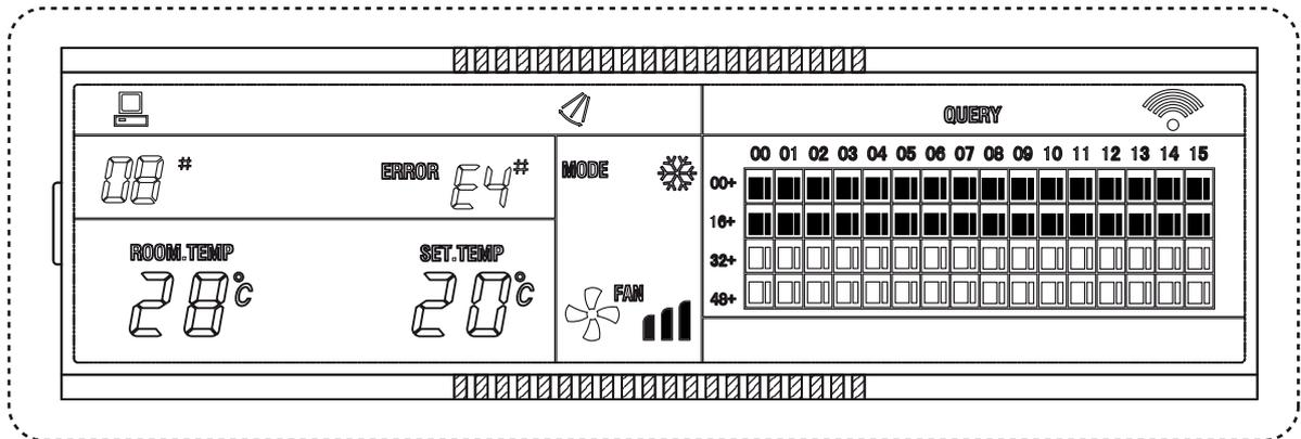
As already observed, each box of the grille is identified by a pair of coordinates, that is by the column number and row number which the box belongs to. In the signal network of DTC-IHXR Centralized Controller, the address of each Indoor Unit is given by the sum of these coordinates. For example, for the Indoor Unit which appears in the box “08, 00+”, the address assigned in the signal network is: 08 + 00 = 08. The screen in “SET” Mode shown above gives the following information:
