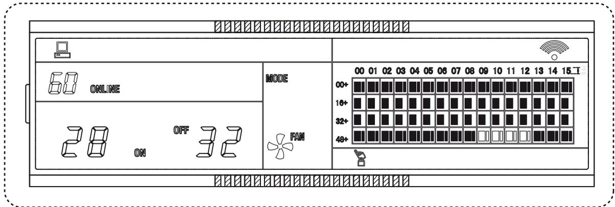
As already observed, each box of the grille is identified by a pair of coordinates, that is by the column number and row number which the box belongs to. In the signal network of DTC-IHXR Centralized Controller, the address of each Indoor Unit is given by the sum of these coordinates. For example, for the Indoor Unit which appears in the box “09, 48+”, the address assigned in the signal network is:  $09 + 48 = 57$ .
